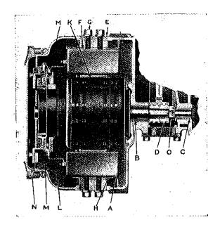
The motor is of the enclosed, fourpole, direct-current series-wound type, with two field coils A; is of the salient pole construction; and lies flat at the side of the compressor. It has no outboard bearing, but has a long liberal bearing B extending into the concave rear end of the armature beyond its centre of gravity, and a smaller bearing C on the inner end of the shaft on the opposite side of the pinion D, so that the latter is not overhung.
